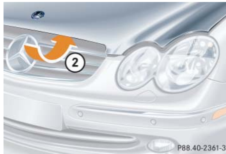
② Lever for opening the hood
